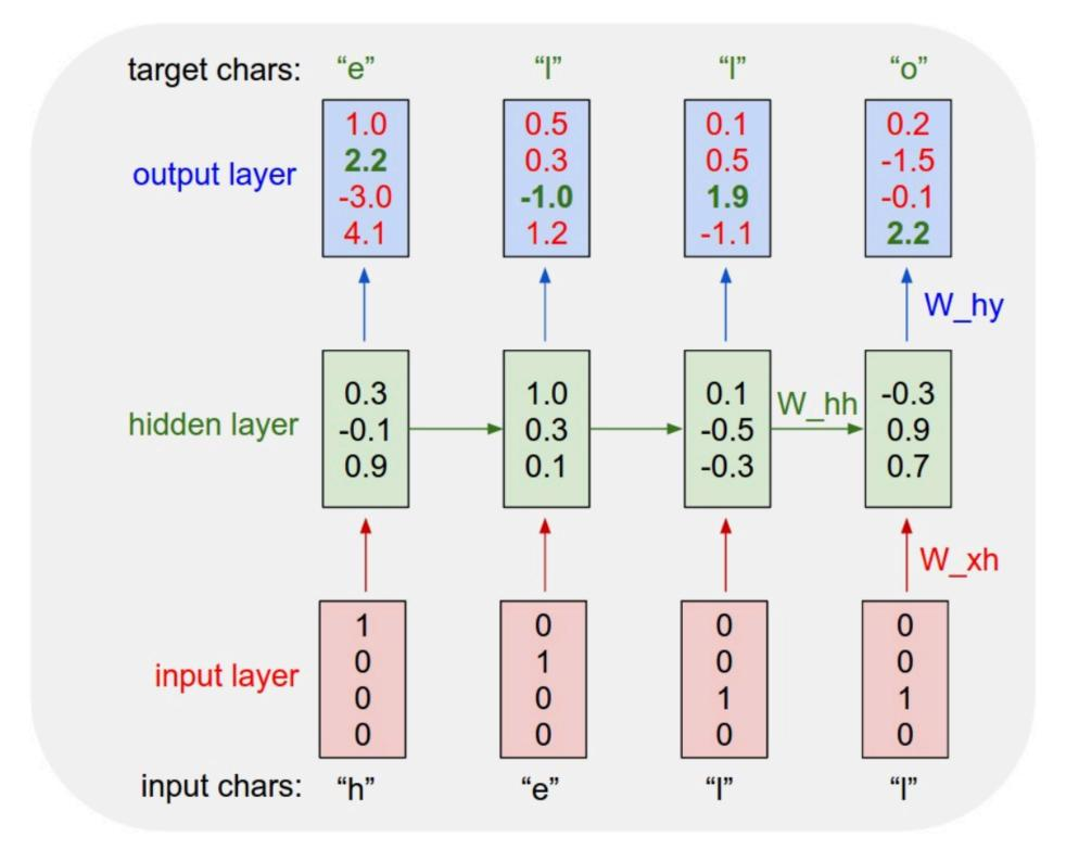
An example RNN with 4-dimensional input and output layers, and a hidden layer of 3 units (neurons). This diagram shows the activations in the forward pass when the RNN is fed the characters "hell" as input. The output layer contains confidences the RNN assigns for the next character (vocabulary is "h,e,l,o"); We want the green numbers to be high and red numbers to be low.
